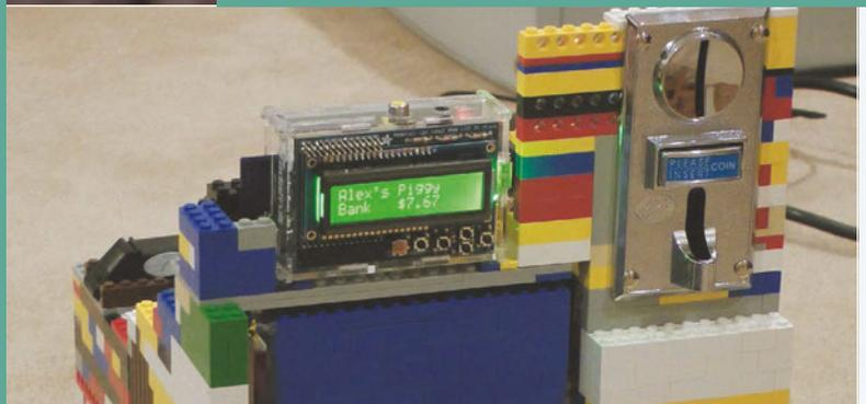
The Raspberry Pi Piggy Bank uses a coin-sorting mechanism to place coins in the correct slots. It counts, sorts and stores coins using a Lego mechanism that rotates for each coin. A fingerprint sensor is used to provide access to the bank.
