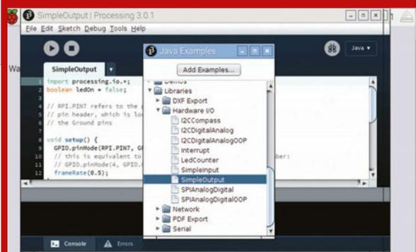
Gottfried’s new Hardware I/O library includes several classes, including those to support GPIO, I<sup>2</sup>C and SPI interfaces. There’s also a PWM class to control hardware pulse-width modulation, and an LED class to flash the Pi’s own built-in LEDs. For more information, see the reference page: [magpi.cc/1XONtQu](http://magpi.cc/1XONtQu)
