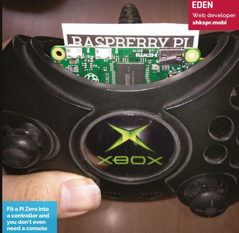
Fit a Pi Zero into a controller and you don't even need a console
