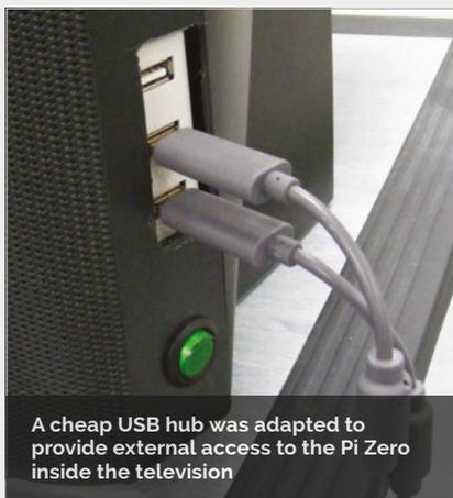
A cheap USB hub was adapted to provide external access to the Pi Zero inside the television
