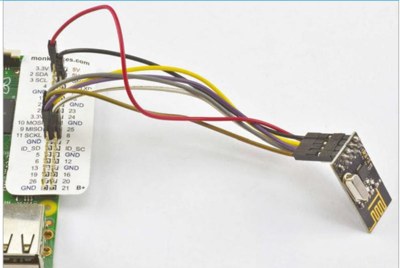
You should wire up the RF module with your Raspberry Pi powered down, and check very carefully that the connections are all correct before you power it back up again. Using a GPIO template like the Raspberry Leaf (by MonkMakes) will help you find the correct connections on the GPIO connector.
