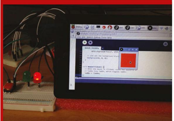
As detailed in the ‘Introduction to Processing’ guide ([magpi.cc/1XOJeEo](http://magpi.cc/1XOJeEo)), a basic example of using the Pi’s GPIO pins with Processing involves lighting an LED whenever the sketch window is clicked (or tapped on a touchscreen). As in Python, the relevant pin is first set as an output, then an if/else block is used to turn it on when the window is clicked – using the GPIO.digitalWrite function to set it to HIGH – and off again when it’s not.
