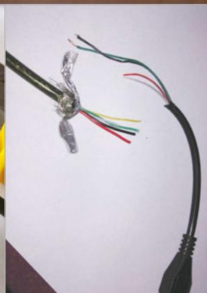
USB OTG is a simple extension to the existing micro-USB spec. The connectors are really cheap: under £1 online. That said, it's pretty simple to make your own if you're confident with wiring and soldering. Terence spliced an old one directly into the controller lead
