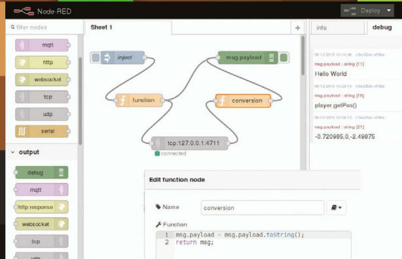
Drag and drop a TCP request node from the function section of the node panel. The server is 127.0.0.1, and the port is 4711. As we're not expecting a return value, we'll Return 'after a fixed timeout' of 0ms. This connects Node-RED to the *Minecraft* TCP socket – if you're keen to understand what a socket is, have a look at the original workshop material: [magpi.cc/1jLWFST](http://magpi.cc/1jLWFST).
