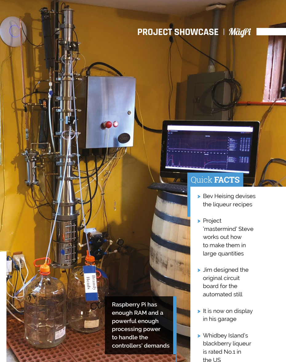
▶ The laptop screen is a convenient way of viewing readings from the still's sensors
