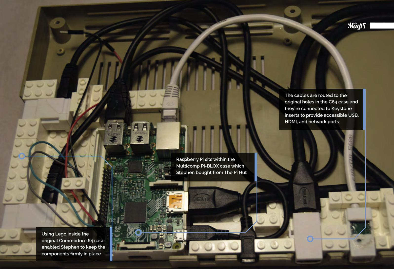
The cables are routed to the original holes in the C64 case and they're connected to Keystone inserts to provide accessible USB, HDMI, and network ports
