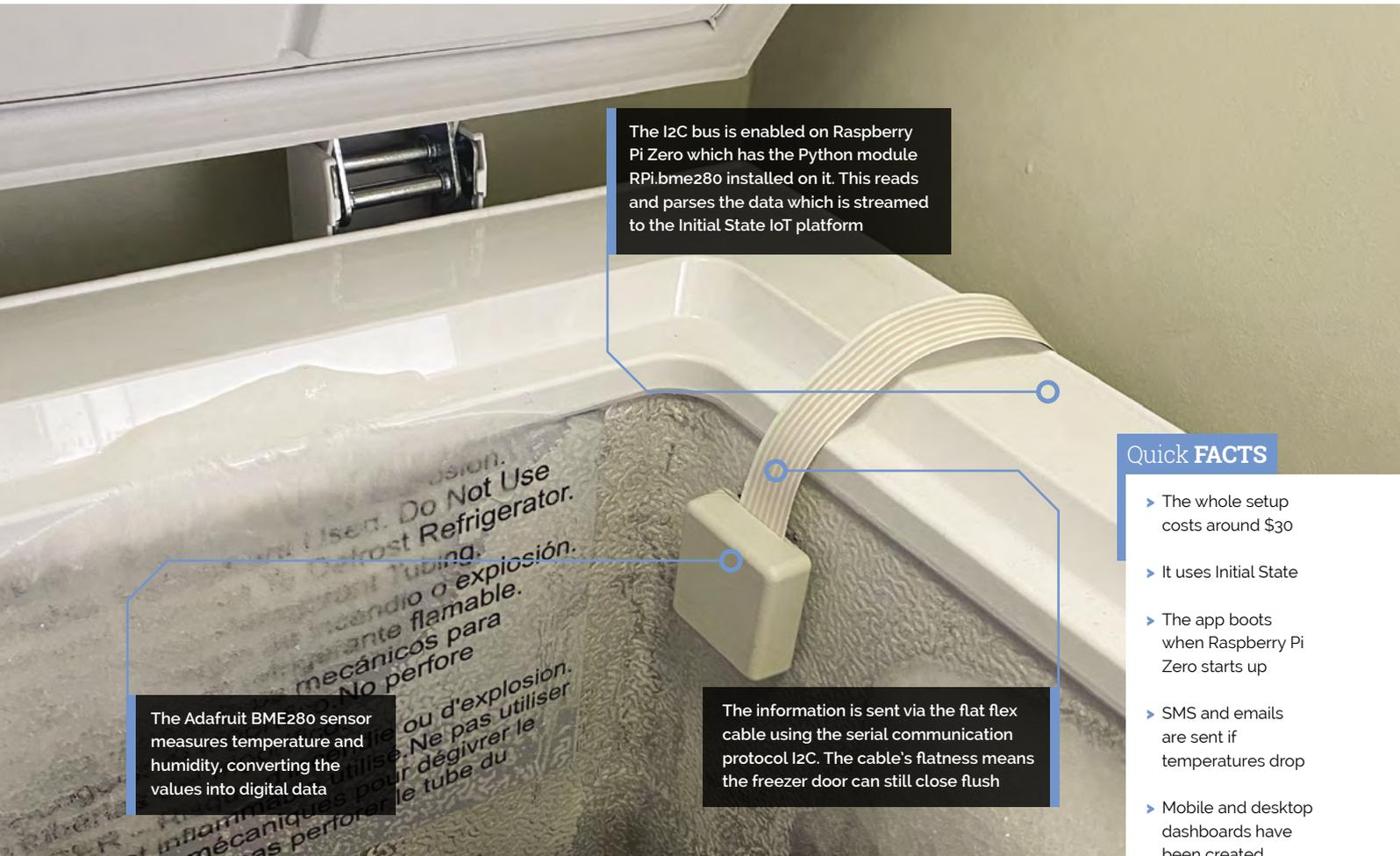
The I2C bus is enabled on Raspberry Pi Zero which has the Python module RPi.bme280 installed on it. This reads and parses the data which is streamed to the Initial State IoT platform
