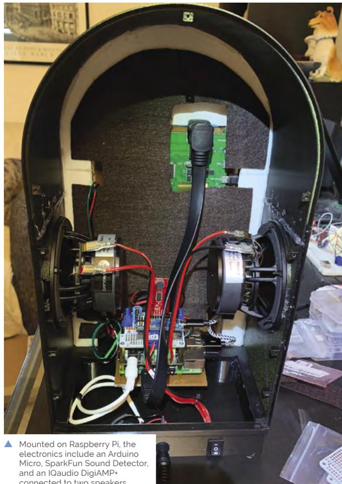
▲ Mounted on Raspberry Pi, the electronics include an Arduino Micro, SparkFun Sound Detector, and an IQaudio DigiAMP+ connected to two speakers
