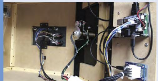
**03** “The workings were simple when it came down to it: Raspberry Pi 3B+ with Pimoroni Picade X HAT. This gives us a power switch, audio amp, buttons, and a joystick if necessary. The replica yoke is interfaced with a USB adapter from the same company. It allows us to use the yoke with the original Atari connector. Software is RetroPie and I'm currently emulating on AdvMAME.”
