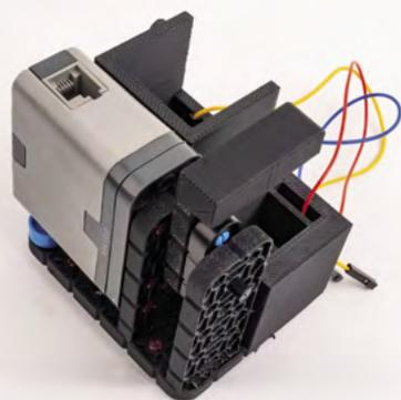
**02** The LED light is sensed by the VEX IQ microcontroller that will move a watering arm over each seedling.
