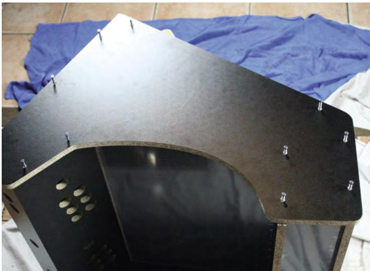
▲ To make it easier to line up the sides of your cabinet with their pre-drilled receiving holes, partially screw in each bolt until a couple of millimetres protrude on the far side
