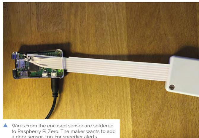
▲ Wires from the encased sensor are soldered to Raspberry Pi Zero. The maker wants to add a door sensor, too, for speedier alerts
