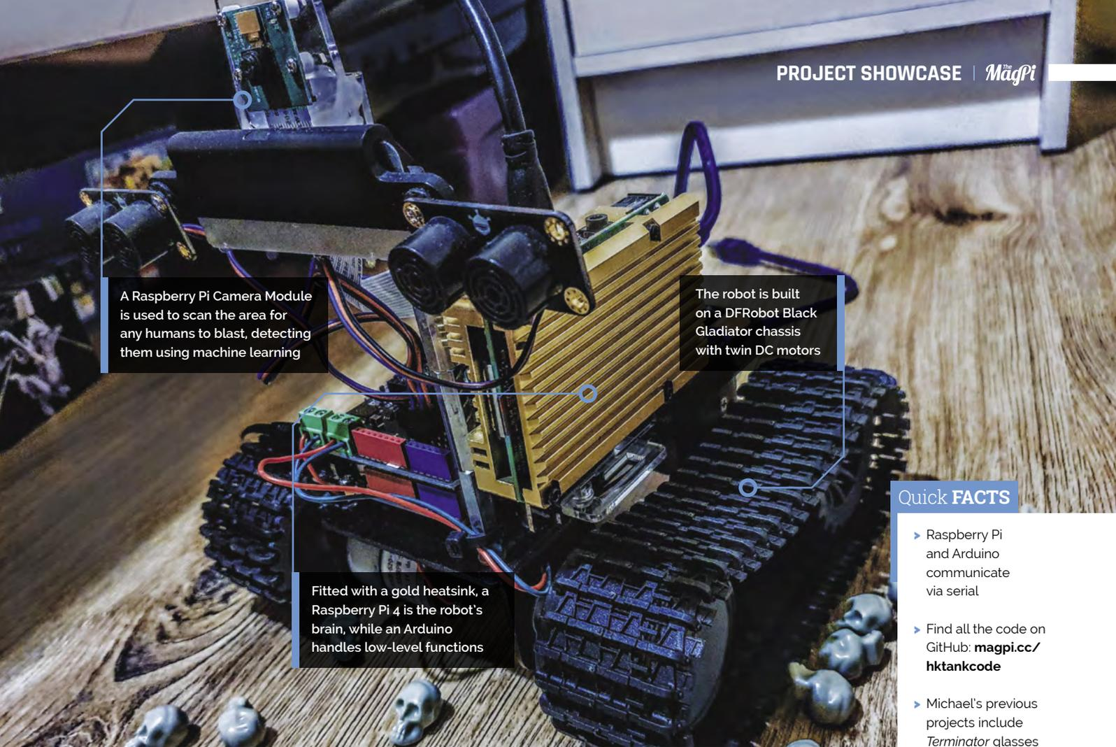
A Raspberry Pi Camera Module is used to scan the area for any humans to blast, detecting them using machine learning
