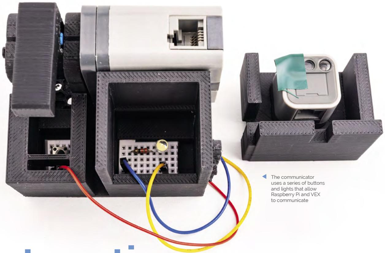
◀ The communicator uses a series of buttons and lights that allow Raspberry Pi and VEX to communicate
