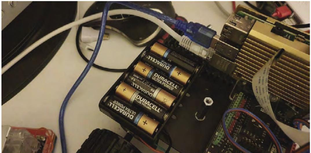
▶ While the Arduino and motors are powered by six AA batteries, a high-capacity power bank is used for Raspberry Pi
