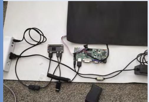
**02** Lay out and connect Raspberry Pi, AV controller board, SD card, and display power cables. A four-gang power strip helps organise power supplies.
