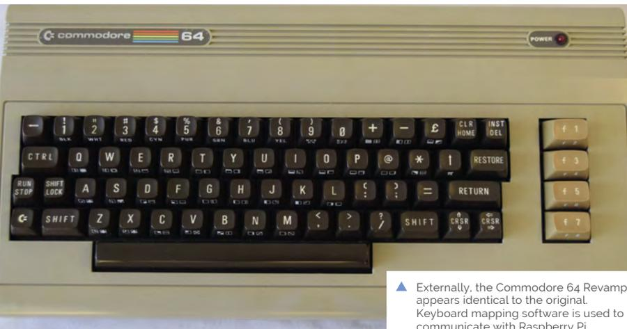
▲ Externally, the Commodore 64 Revamp appears identical to the original. Keyboard mapping software is used to communicate with Raspberry Pi
