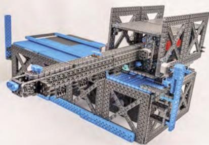
**03** As the arm is over a seedling, the VEX IQ microcontroller pushes a button that is sensed by Raspberry Pi and triggers a watering pump to stream water over the plant. The apparatus does this for each plant and then resets.
