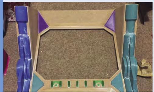
**02** The cabinet was designed and laser-cut from MDF. There's some steel in the construction, as well as tempered glass over the screen. Mouldings are 3D-printed, with the help of a graphic artist who also helped rework graphics to fit the smaller size. Lastly, a riser is constructed to make sure it's tall enough to play.
