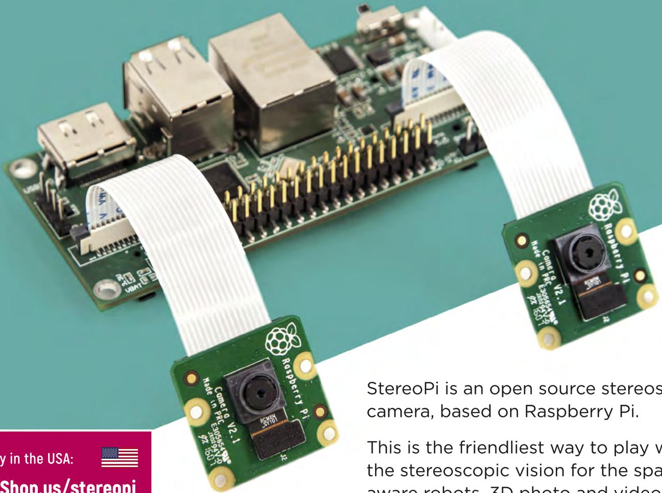
StereoPi is an open source stereoscopic camera, based on Raspberry Pi.
