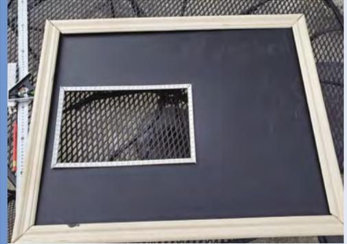
**01** Setting up an LCD chalkboard is broadly similar to creating a magic mirror, for which detailed instructions are on GitHub ([magpi.cc/magicmirrorgit](https://magpi.cc/magicmirrorgit)). Apply chalkboard paint to one side of your plywood chalkboard, then cut out a hole the correct size and dimensions for your LCD. Measure and fit the frame.
