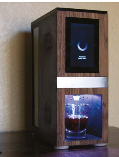
▲ There is some splashing, but Pegor believes a longer nozzle will fix this
