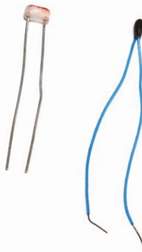
◀ Figure 5 The light-dependant resistor and thermistor can be used to measure analogue light and temperature levels
