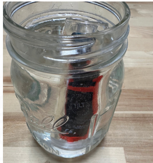
▲ Step 02: Submerge Tilt while powering it up
