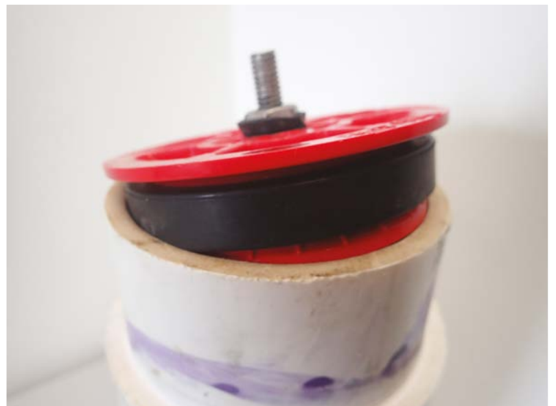
▲ The seal uses a very simple plumbing system
