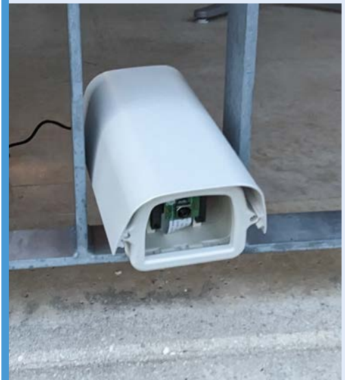
▲ Raspberry Pi is protected inside a waterproof case
