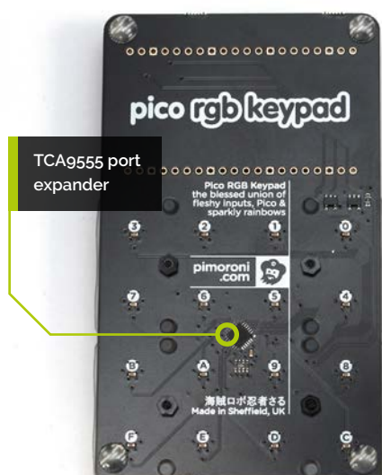
▲ Figure 4 The TCA9555 port expander is the small square integrated circuit mounted on the rear of the keypad PCB
