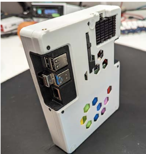
▲ The Raspberry Pi computer ports can be accessed from the back. There's also a kickstand, power switch, and accessory mount
