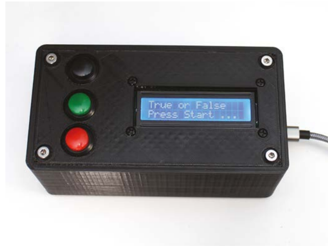
▲ Figure 7: The game can be placed inside an enclosure. If you don't have a 3D printer, you can use a generic case and cut appropriate holes
