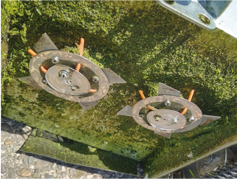
▲ An underside view of the robot shows its two rotary blades which enable pebbles to be ejected
