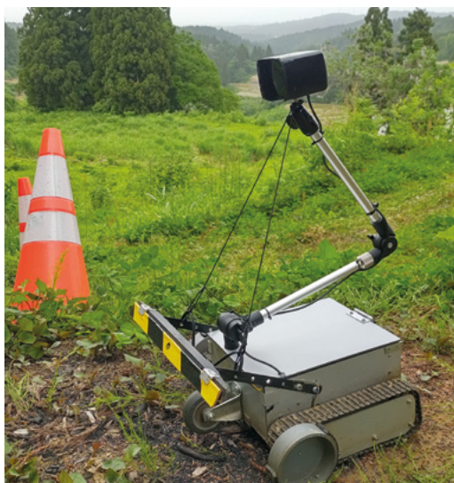
▶ Traffic cones act as a visual guide for Roktrack, helping it to work its way around an identified area
