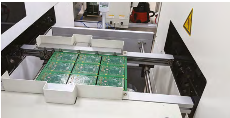
▲ Sheets of naked Raspberry Pi 4, ready to be assembled
