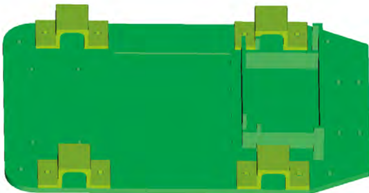
Figure 1: Robot chassis design created in FreeCAD. Includes four motor brackets which are printed separately
