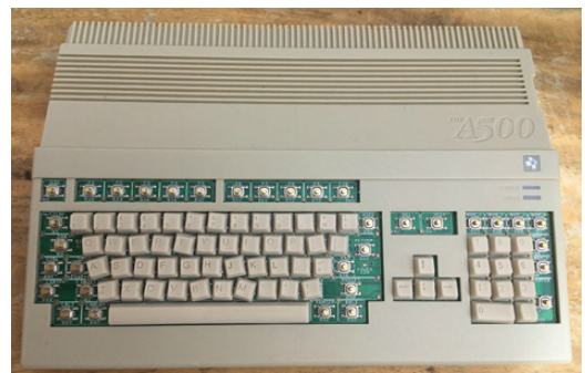
▲ The keys were twisting out of alignment, and Dean found oval switches were the best solution
