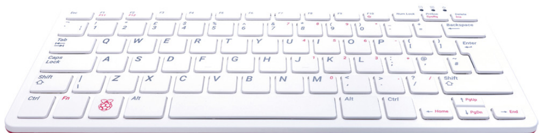
► Figure 17: Raspberry Pi 400 has an integrated keyboard
