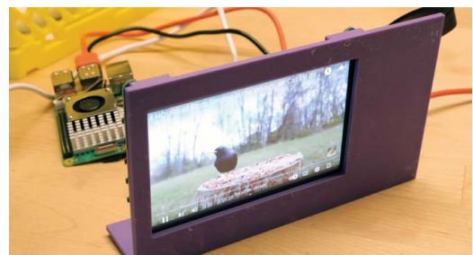
▲ Raspberry Pi Zero and an Elecrow touchscreen form the project's basis, all wrapped in a custom enclosure
