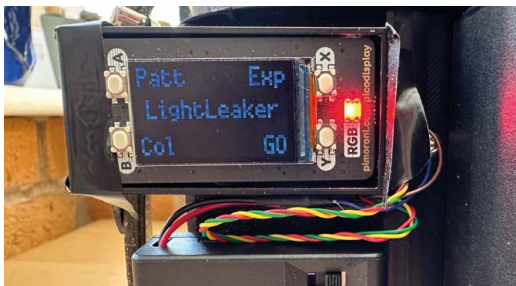
Figure 9 ♦ You select a particular function by pressing the name next to it. The middle of the display is used for messages
