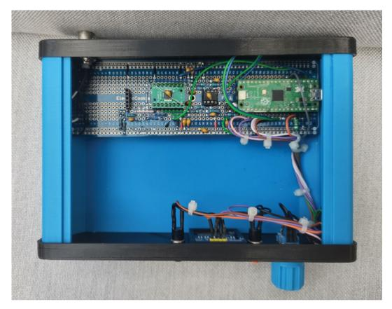
desired listening frequency, generated by Pico's PIOs, the multiplexer switches the incoming radio signals rapidly between four paths. These samples are then combined and amplified in the dual op amp to generate lower-frequency I and Q (in-phase and quadrature) signals that can be sampled using the analogue-to-digital converter in Raspberry Pi Pico.
