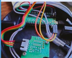
Raspberry Pi Pico inside the Gesture Controller is attached to an AHRS IMU sensor (which detects the pedal's movements) and via USB to a PC where it can act as a MIDI control device.
