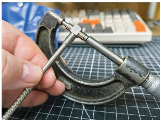
Using the tool isn't really that difficult, but you need develop a consistent technique so that you can get repeatable results. Begin by inserting the telescoping gauge into the space that you're trying to measure, with the nut loose so that the sprung probes are free to snap to each side of the space.
