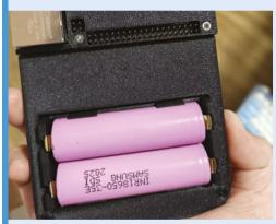
This model is not going to be powered by Nokia batteries. Instead, a pair of rechargeable 3500 mAh-capacity batteries with a nominal voltage of 3.6V are going to be used. Again, this will increase the bulk. A new battery housing has been created.
