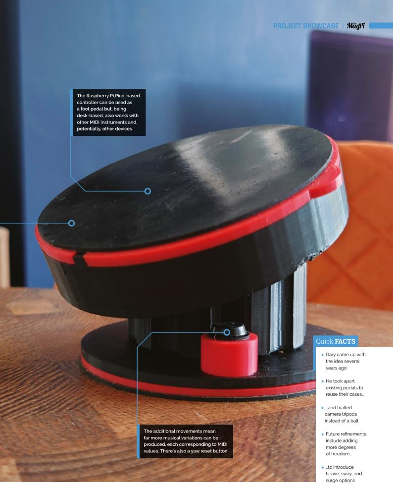
values are sent down a serial line, so the Gesture Controller could theoretically be used in "any situation needing a multi-axis controller".
