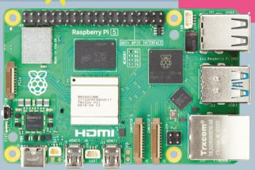
To fit all of Raspberry Pi 5's goodness in a much smaller footprint, the CM5 copper layers rather than the six on Raspberry Pi 5
