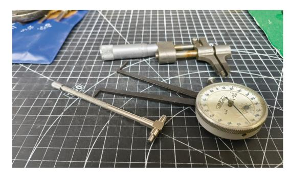
elescopic gauges are a great way to start an argument between professional machinists. They're a tool for measuring interior diameters, so you'll mostly use them when you're trying to measure the diameter of a bore or slot. In this article you'll see what the fuss is all about, and learn how to properly use a telescopic gauge.
