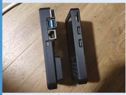
Zitao is now developing a new version of the Hackberry Pi which will use a Raspberry Pi 4 computer rather than Raspberry Pi Zero 2 W. As you can see, it will make for a far chunkier device and fresh design decisions need to be made.
