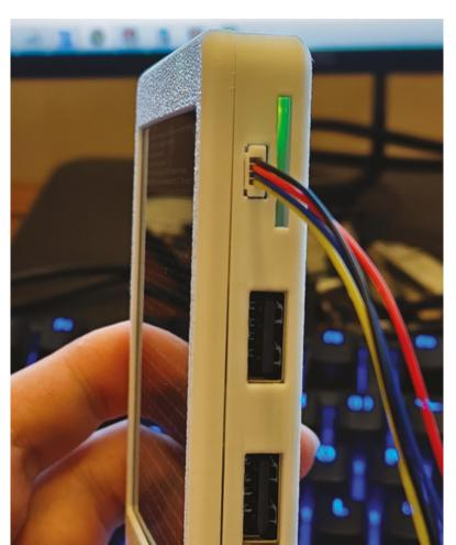
A STEMMA QT port has been added, accessible from the right-hand side. It allows breakout boards and sensors to
